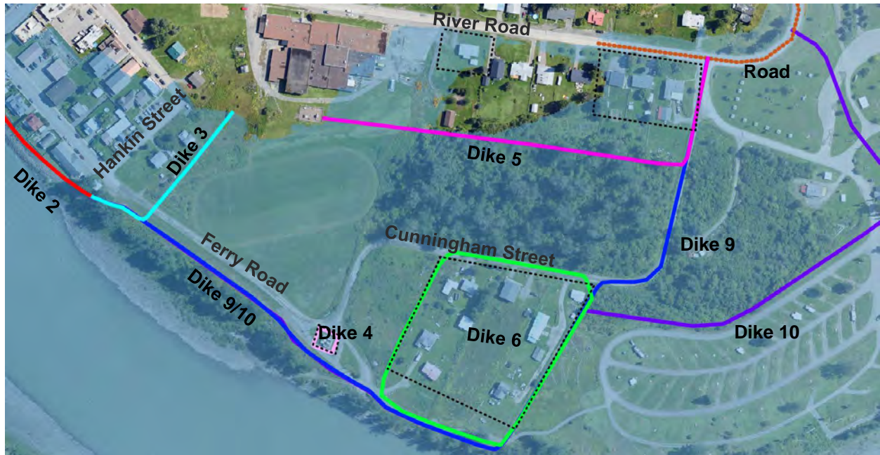
Figure 5-5: Dike Options Considered and Approximate Buildings in Inundated Area (Dashed Black Line) for Zone 3 and Zone 4.
