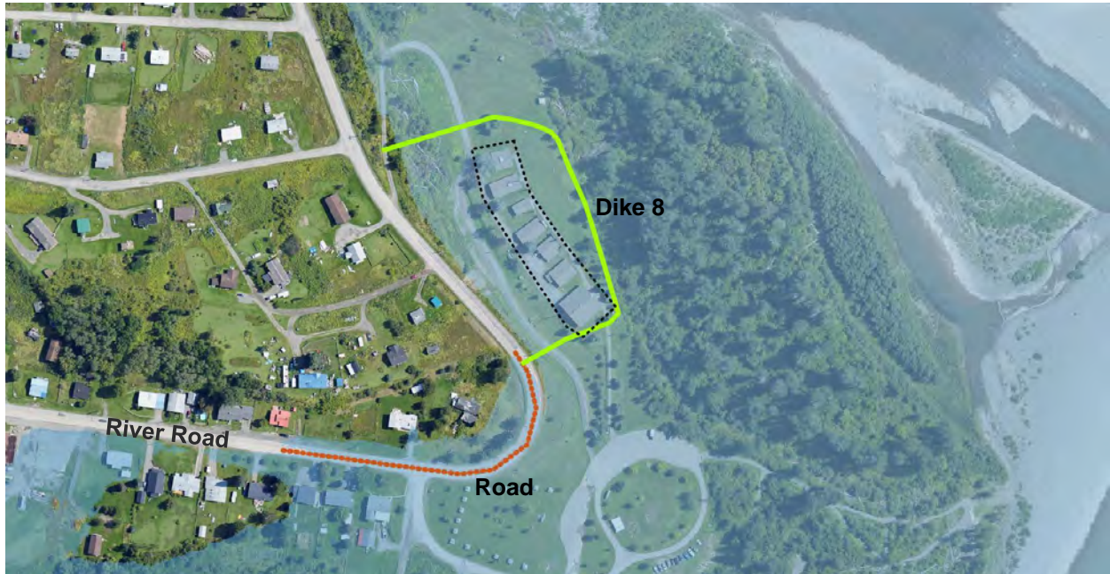
Figure 5-7: Dike Option Considered and Approximate Buildings in Inundated Area (Dashed Black Line) for Zone 6
